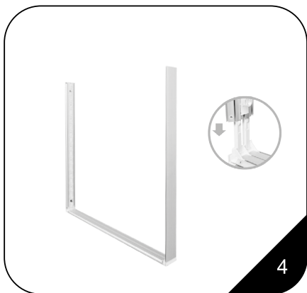
Assemble the top half of the frame by connect the parts with matching numbers
